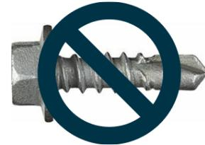
*\* The Tri-Fixx M8 heavy duty screw needs to be drilled at a slower speed of less than 100rpm in order for the screw to start cutting the steel - high speed drilling of this screw will only heat treat the steel making it impossible for the screw to penetrate the steel.*
