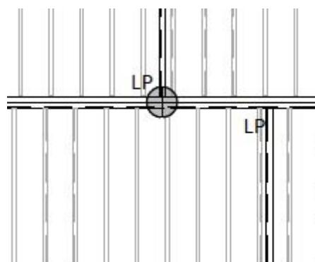
**FIX:** Engineer to reposition piles away from the edges and joists to avoid this clash or avoid the use of the backing plate as detailed below.
